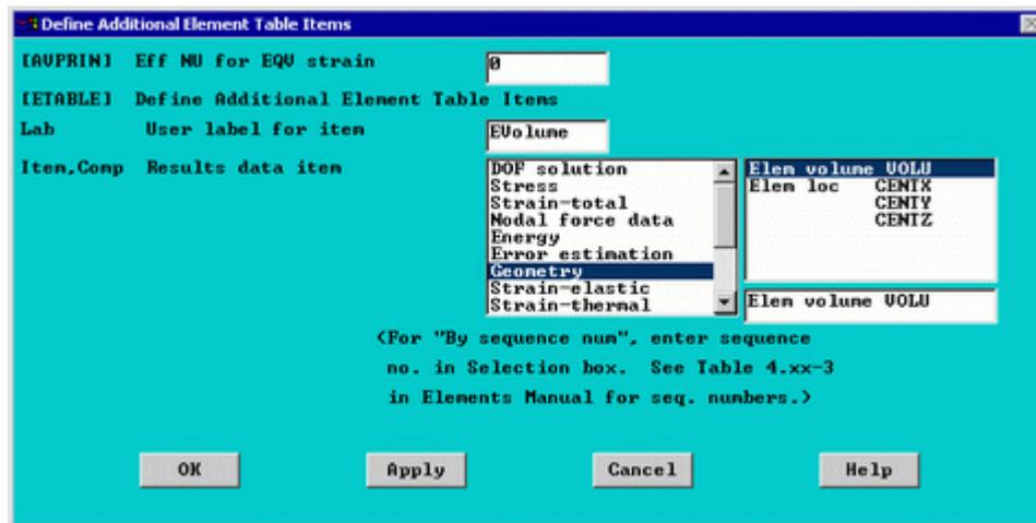
Note that this is the volume of each element. If you were to list the element table you would get a volume for each element. Therefore, you have to sum the element values together to obtain the total volume of the beam. Follow the instructions below to do this.
