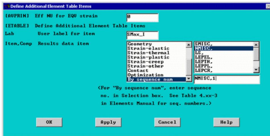
Note that nmisc,1 is the maximum stress. For further information type `Help beam3` into the command line
